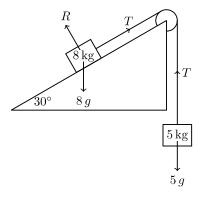
Students were expected to label the two weight forces, the normal reaction force on the 8 kg mass and the tension force in the string.
