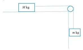
The diagram above shows a light inextensible string that passes over a smooth pulley and connects a body of mass M kg sitting on a rough horizontal plane to a body of mass m kg, which is hanging vertically. The coefficient of friction between the body of mass M kg and the plane is  $\frac{1}{3}$ . When the system is released from rest, it accelerates at 2 ms<sup>-2</sup>.
