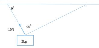
The diagram above shows a string is attached two points on a horizontal ceiling. A 2kg mass is tied to the string so that a right-angle is formed. If the tension in one section of the string is 10N, then angle that  $\theta$  that this string makes with the ceiling is closest to
