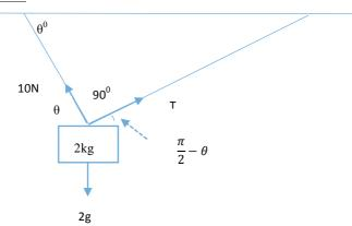
Let the angle made between the string and the ceiling be  $\theta$  and the tension in the other section of the string be T.
