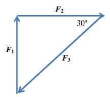
$$\frac{F_1}{\sin 30^\circ} = \frac{F_2}{\sin 60^\circ} = \frac{F_3}{\sin 90^\circ}$$
