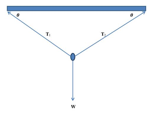
An object in **equilibrium** is suspended from a beam by two ropes, each making an angle of  $\theta$  with the horizontal. The tension forces acting on the object are  $\mathbf{T}_1$  and  $\mathbf{T}_2$  and  $\mathbf{W}$  is the weight force. Which one of the following statements is true?
