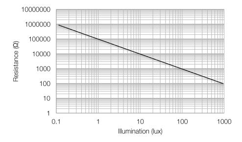
The switching circuit will turn the light on when it is connected to a voltage equal to or greater than 8.8 V. Tom notices that when the illumination equals 10 lux, the light turns on.
