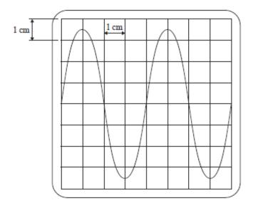
The vertical scale is set to 2.5 V/cm and the horizontal scale is set to 5 ms/cm.
