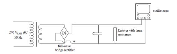
He uses the oscilloscope calibrated in the same way as questions 9 and 10: the vertical being  $2.5 \, \text{V/cm}$  and the horizontal being  $5 \, \text{ms/cm}$ .
