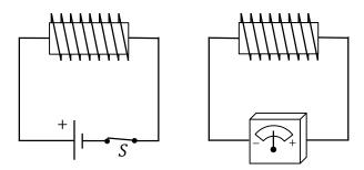
Initially, switch S is closed and the current through the electromagnet is 0.5 A.
