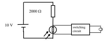
Common errors included placing the switching circuit in series with the battery, resistor and LDR. This was unusual given the relatively standard circuit design required in this type of circuit. Another common error was connecting the switching circuit in parallel with the resistor.
