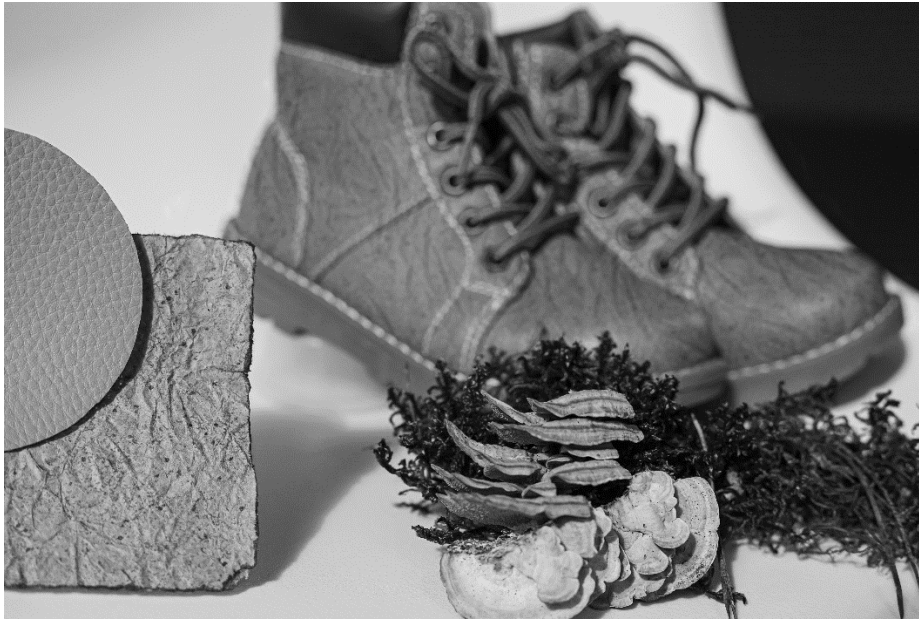
Vegan leather shoes from mushroom mycelium and samples of vegan bio leather.
