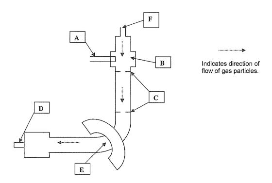
The diagram shows a simplified cross section of a mass spectrometer.
