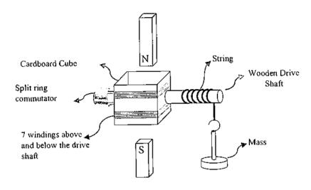
The student is disappointed to see that, although the motor rotates with no frictional effects, it cannot lift a mass of more than 20 g even on the highest power setting.
