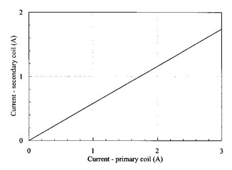
If there are 580 turns in the primary coil, the number of turns in the secondary coil is closest to
