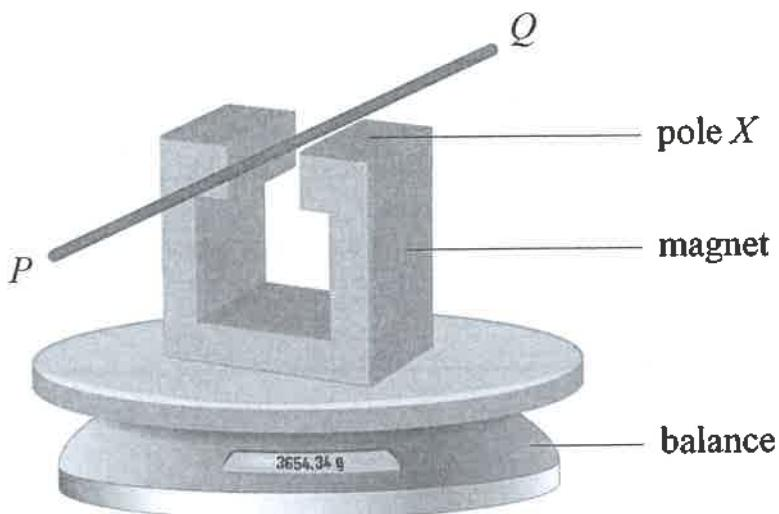
When a direct current of 3.2 A is passed through the rod from  $P$  to  $Q$ , the reading on the digital balance increases by 2.69 grams.
