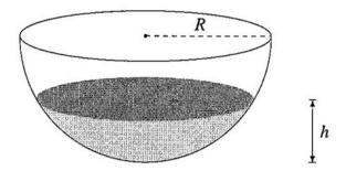
A bird bath of radius 0.5 m is being filled with water at a constant rate of 0.03 m<sup>3</sup>/minute. Calculate the exact rate at which the height of water is increasing when h = 0.25 m.
